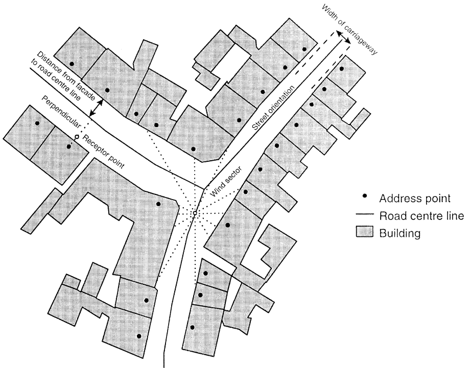
Fig. 2. Street configuration parameters generated by the urban landscape model for use in the OSPM to calculate air pollution levels. The digital map includes building polygons, address points and polylines to represent the middle of roads.
